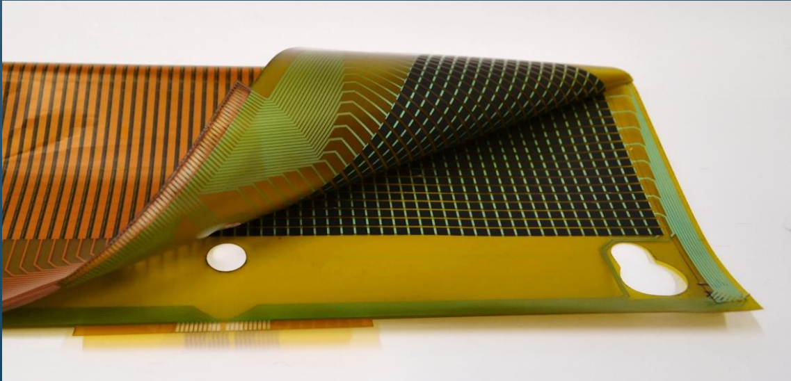
Matrix of printed piezoresistive pixels on thin polyimide substrate.
